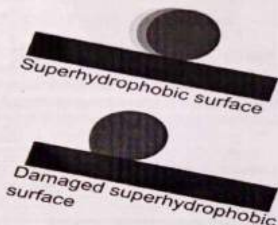
Figure 4. Due to the high contact angle and low hysteresis, water droplets easily roll off super hydrophobic surfaces. However, damage to the surface often leads to an increased contact angle hysteresis and, consequently, droplets stick to the surface.
